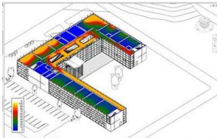
Fig: Daylight Analysis for Revit on Autodesk Labs
